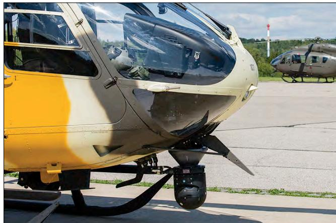
Close-up showing the FLIR installation, which is only fitted to the aggressor Lakotas, on UH-72A 09-72107. (25 August 2021)
