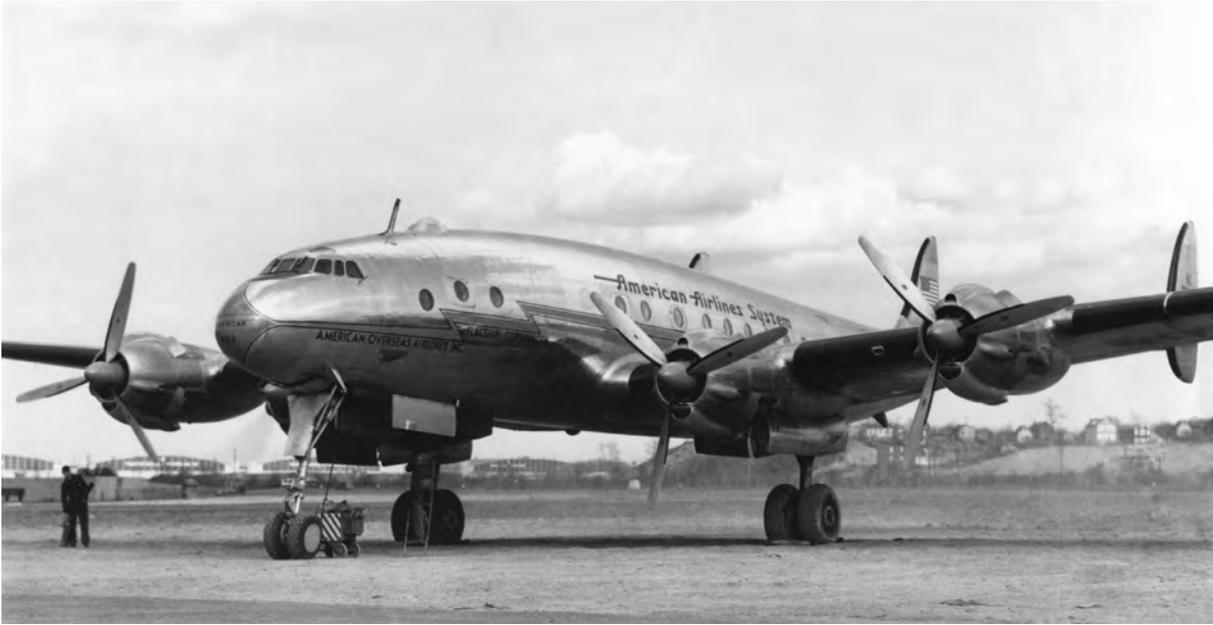
This Lockheed Constellation was the earliest version of the civilian Connie, the L-049. It can easily be distinguished from the later L-749 versions by the presence of exhaust stacks in the side of the NACA cowlings. The L-049 on photo, N90922 (2052) was delivered to American Overseas Airlines on 25 March 1946 as
