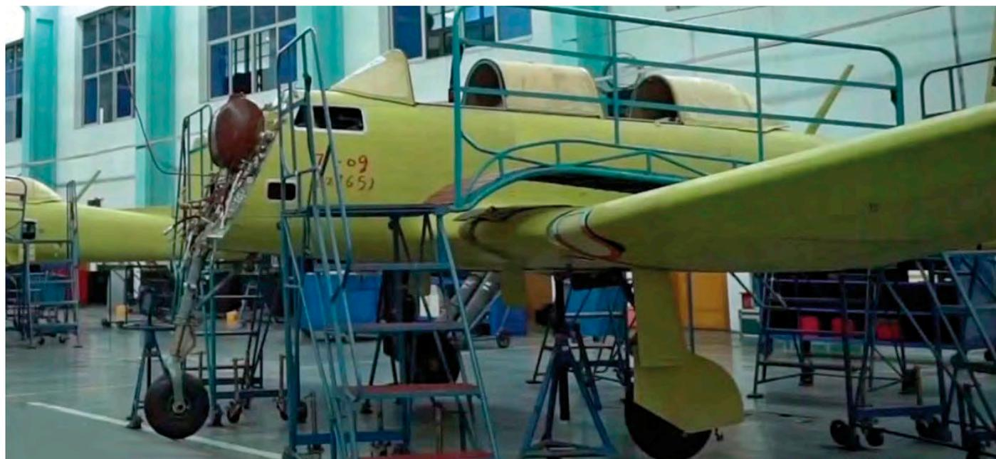
*Some unique footage taken after the re-opening of the Hongdu production line disclosed these numerals crudely scribbled on the nose in red on this primer CJ-6A. It reads '71-09' and '2765', the 2765th CJ-6 built, batch 71, sequence number 09. (aired 1 April 2018, CCTV7)*
