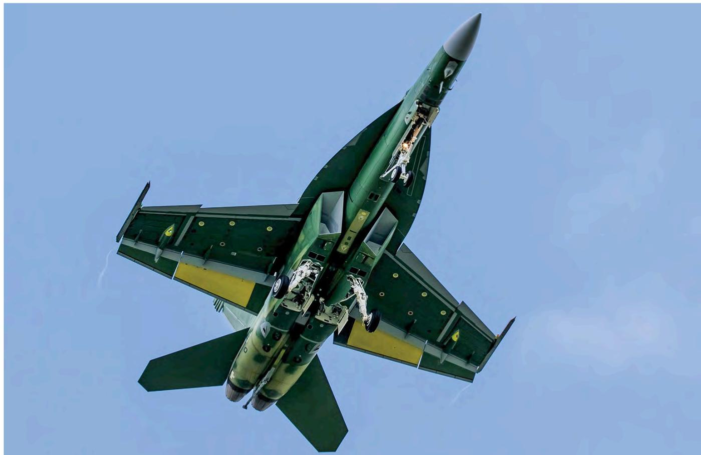
Captured on final of Lambert-St. Louis International (MO) after a testflight is F/A-18F 169751, the first Block III Super Hornet. This new version is capable of carrying shoulder-mounted conformal fuel tanks, among many other system improvements. (May 2020, Chase Kohler)
