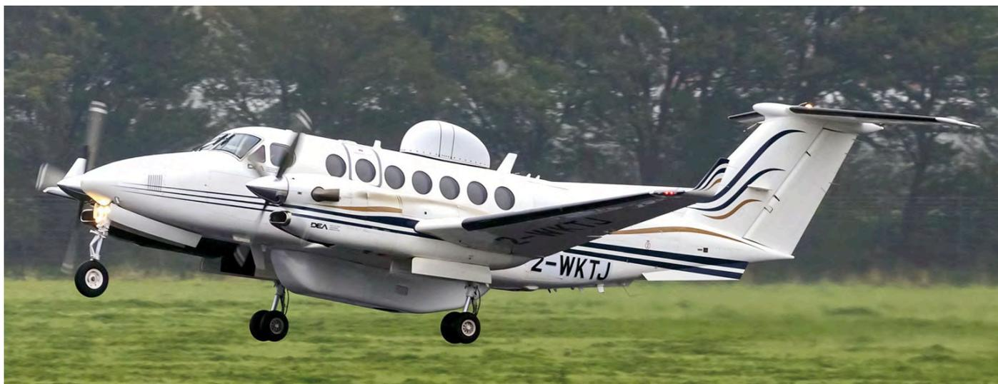
This Super King Air 350 2-WKTJ (with msn FL-470) was registered into the register of Guernsey in October this year and is operating for Diamond Executive Aviation. This aircraft has been used since as an airborne relay- and measurement aircraft, as can be seen by the extra dome on top and extra belly under the fuselage. (Rotterdam - The Hague, 1 November 2019, JvL.Holland)
