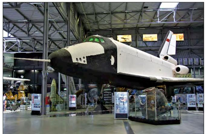
Though built as a spacecraft, one Buran was equipped with jet engines to enable autonomous test flights, and so became an aircraft. Uniquely marked as CCCP-3501002, it has been on display in Australia, stored in Bahrain and eventually preserved at the Technik Museum Speyer. (7 September 2019, Raymond van Dijkhuizen)
