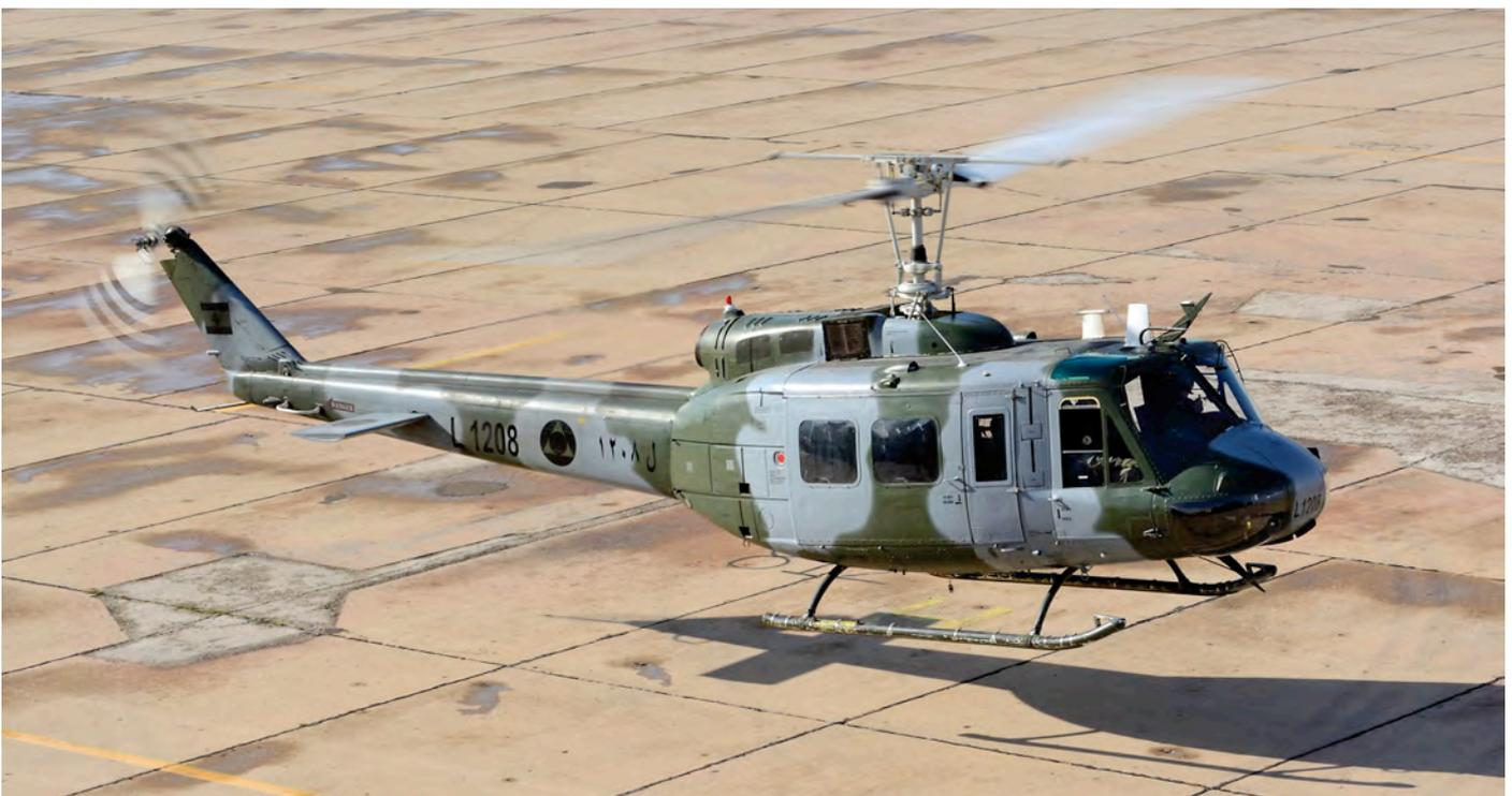
*The latest incarnation of the faithful Huey is the Huey II. Equipped with the transmission of the Bell 212 and with a higher rated engine, this has rejuvenated the proven design and they are set to be around for a while yet. After being used in mix with the UH-1H, all Huey IIs are now nominally on 12sq strength; although one was with the Kleyate delegation too.*
