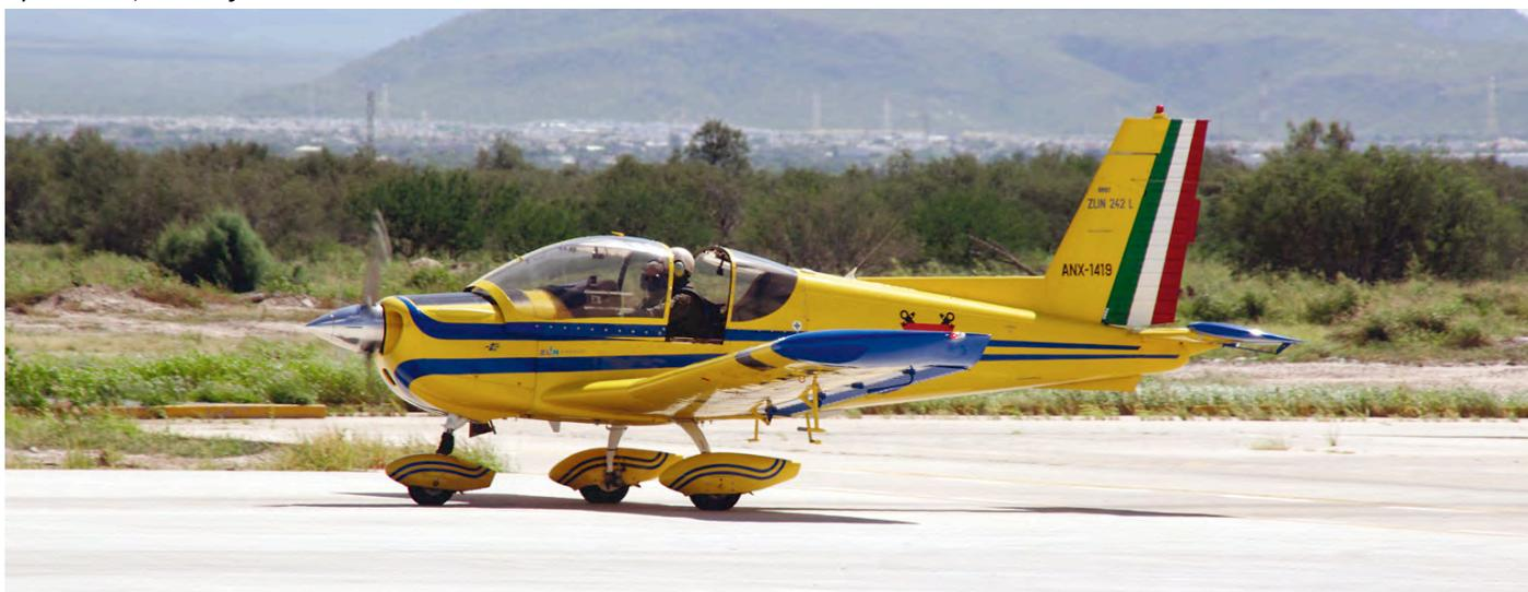
The Zlin 242L has some distinctive features like landing gear sockets and a forward sliding canopy. The latter comes to good use before and after a flight in the hot conditions in Baja California Sur!
