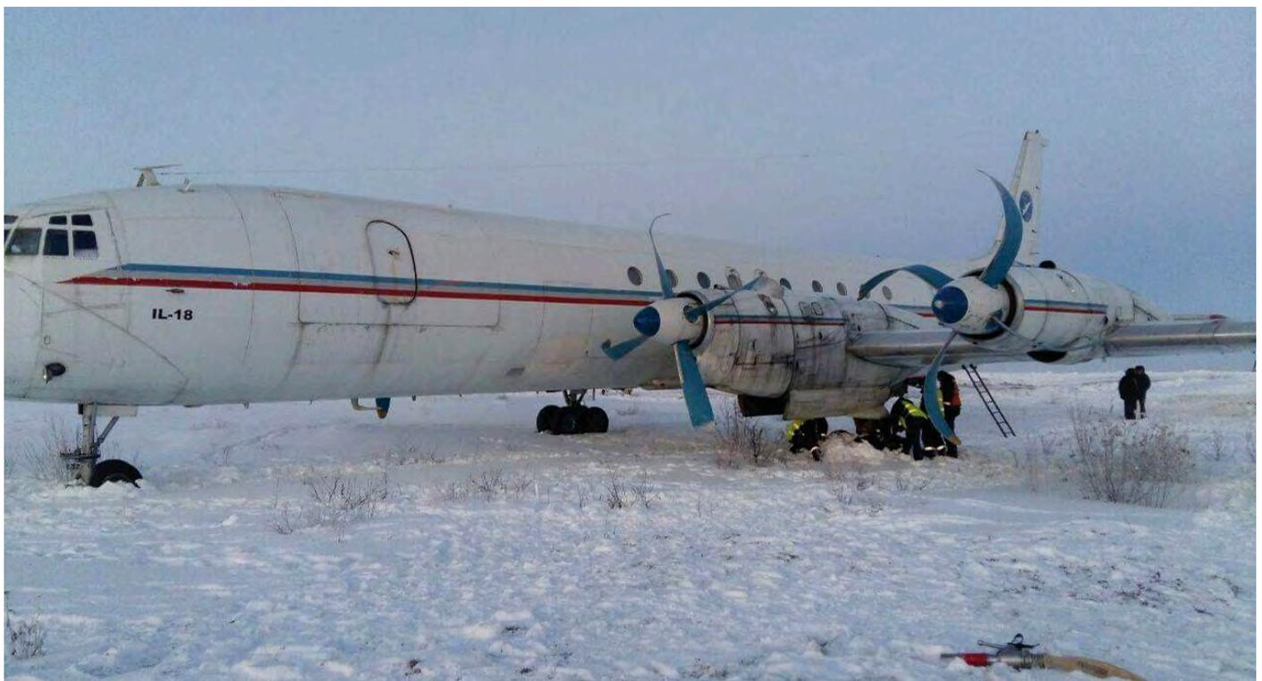
Il-18Grm 54006 of NPP Mir suffered a runway excursion after landing at Naryan-Mar Airport, Russia, after a flight that started in Syktyvkar Airport. The aircraft came to rest in the snow, past the runway end. The propeller blades suffered damage during the overrun, the cause of which is to be determined. (Credit info Alex Snow)
