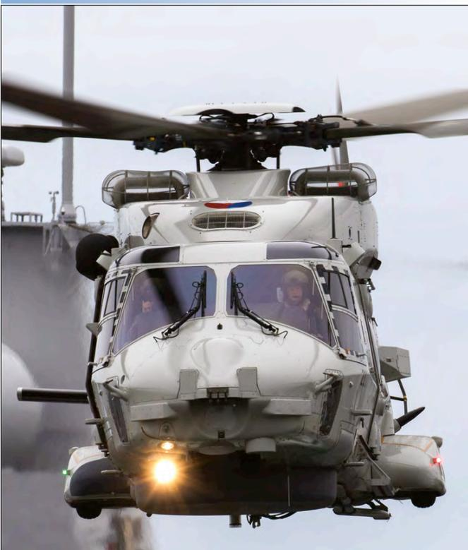
Sander Meijering captured N-233 during the Navy Days in Den Helder on 24 June 2017. This NH90-NFH is a de-scoped version, noticeable by the missing FLIR, lack of sensor bulbs and missing cable cutter above the cockpit.
