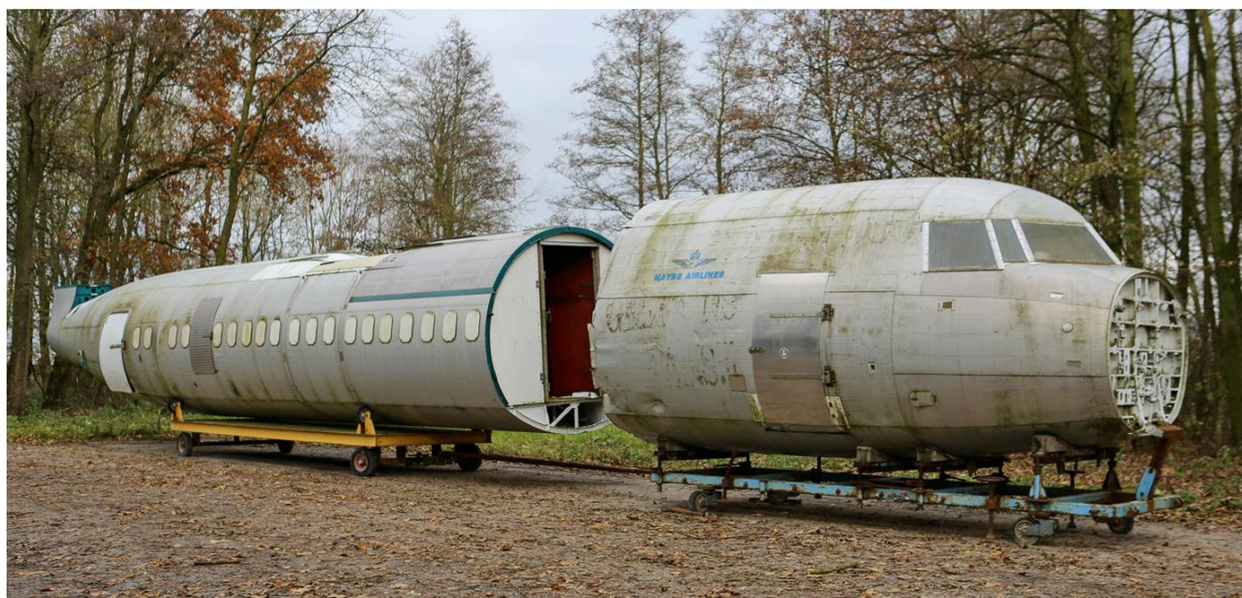
The fire brigade at Lelystad airport is using two parts of unfinished Fokker 50s. The nose section is part of c/n 20318 and the fuselage section is part of c/n 20325. Both are so-called "FNB's", also known as "Frame Not Built". (Lelystad, 1 December 2016, Berend Jan Floor)
